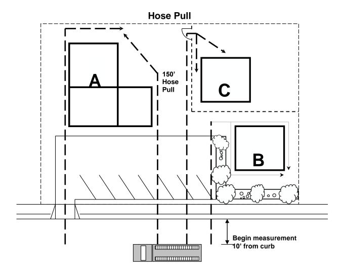
In the example above, assume that the parking lot is not accessible to fire apparatus due to turning radii and fire lane widths less than the required minimums.
