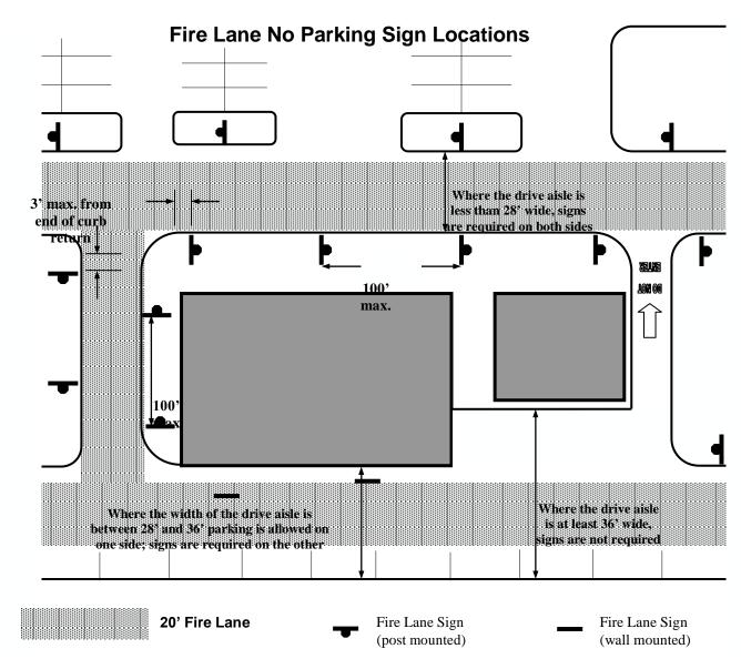
Signs are required within 3' of the end of the curb return at the beginning of each "block" along the fire lane and spaced a maximum of 100' along the entire designated lane. A sign shall be located within a reasonable distance of the end of each block as necessary to clearly identify the extent of the no parking zone. One sign is required for each island adjacent to the fire lane that is large enough to accommodate a parked car.
